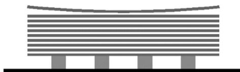
Figura 1.15 – Empeno do painel superior
